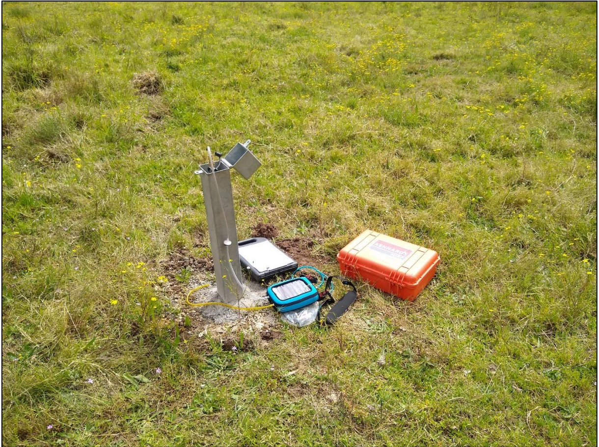
Figure 7: Gas monitoring set up
