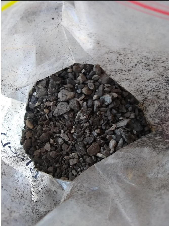
Figure 8: Carbonaceous seams within sandstone bedrock (Bore 6001)
